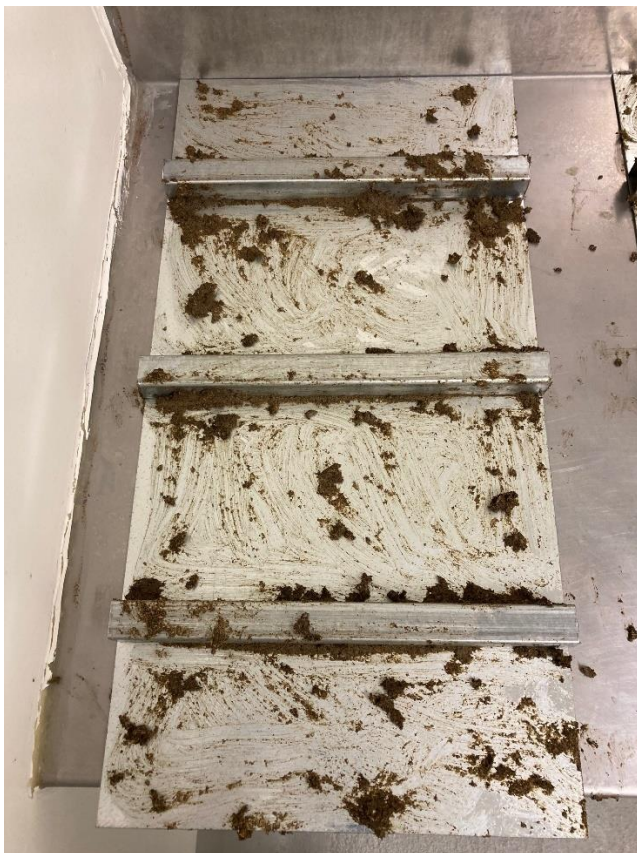
Figure 2: Mock truck tray floor after being smeared with 100 g of faeces.
